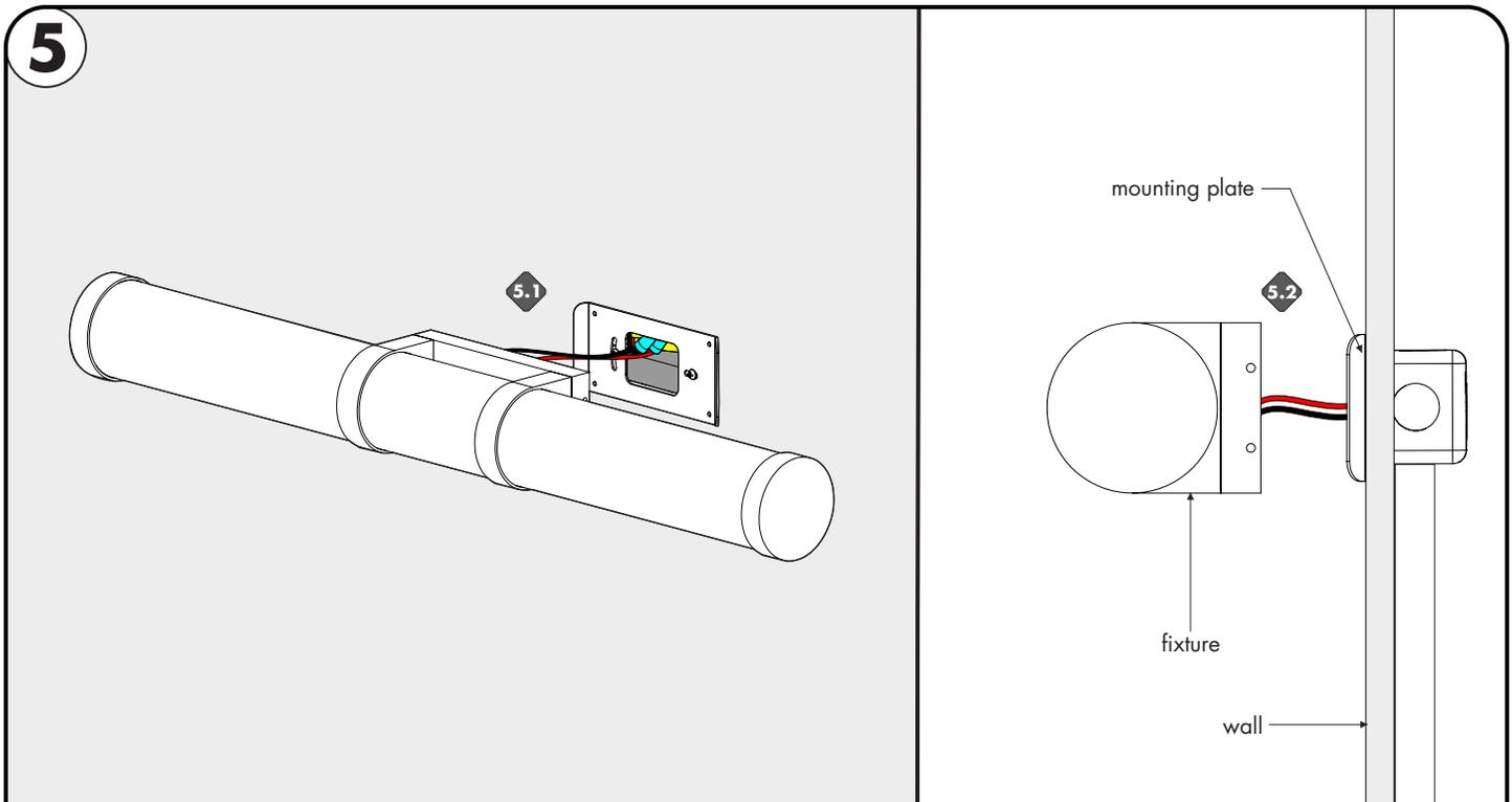
**5.1** Insert the fixture wire nut connections into the junction box.
