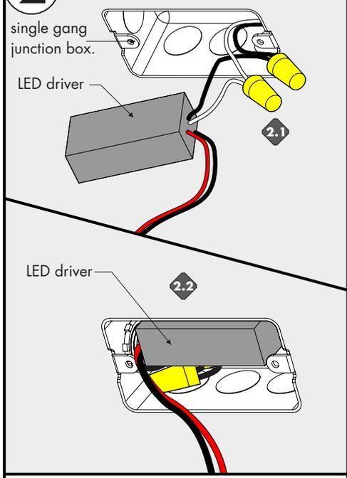
**2.1** Connect the white (neutral) & black (hot) LED driver wires to the white & black power wires (120VAC).
