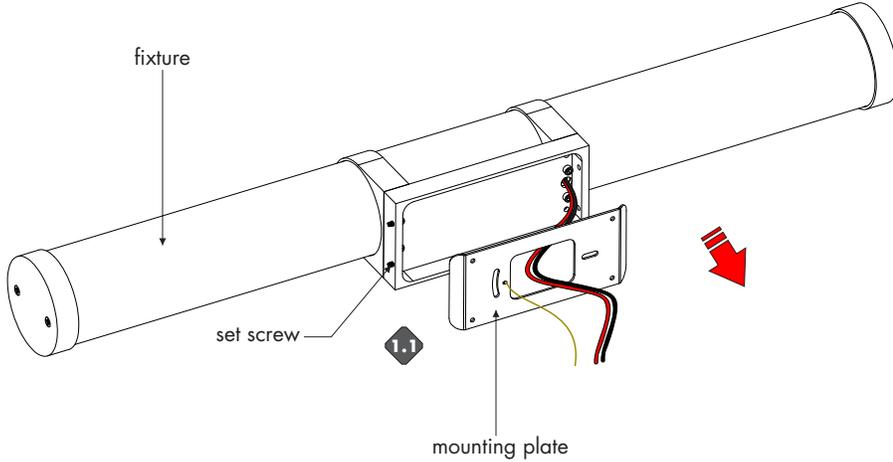
**1.1** From the back of the fixture, loosen the 4 set screws on the fixture body. Then carefully remove the mounting plate.
