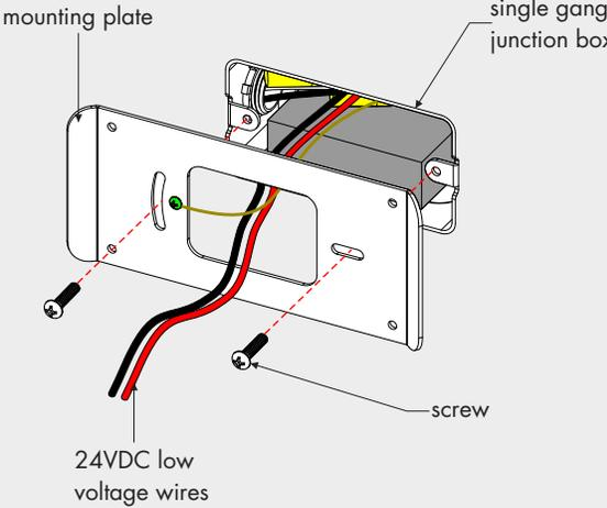
**3.1** Feed the low voltage wires through the center of the mounting plate. Followed by lining up the mounting plate to the junction box and secure using the provided screws.
