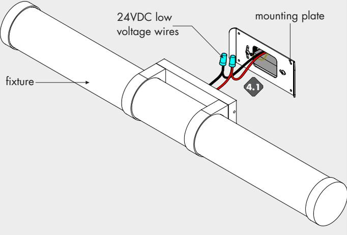
**4.1** Connect +24 VDC red wire from the fixture to the LED driver +24 VDC red wire with a wire nut. Connect -24VDC black wire from the fixture to LED driver -24VDC black wire with a wire nut.
